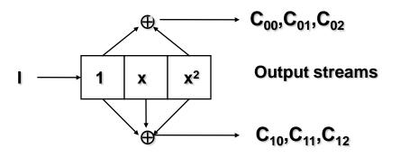
For encoding of convolution codes so called
