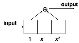
will multiply the input stream by  $x^2+1$  and the second shift register
